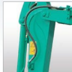
Auxiliary Hydraulic Piping
